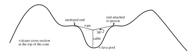
1b. The actual apparatus has a pulley in the middle of the rope. The cable parallels one side of the rope, goes over the pulley and down to the lava pool. The reason for this is that simply tightening the rope can't lift the lava sample out. Here's why: calculate how much tension would be needed in the rope to decrease the angle to  $5^{\circ}$ .
