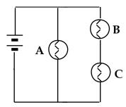
5. In the circuit above, how does the flow rate through A compare to that through B? How many times brighter should A be compared to B? Explain.
