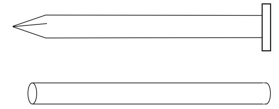
2. Now the nail and the rod are separately brought near (but NOT in contact with) a negatively charged Van de Graaff generator. For each object, explain and sketch the changes in the distribution of the charged particles.
