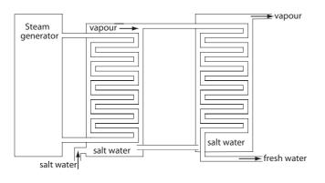
Figure 1621 The Distillation process
