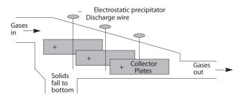
Figue 1607 The principle of electrostatic precipitation
