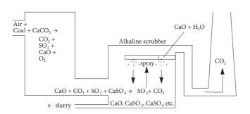
Figure 1606 The principle of a 'wet scrubber'
