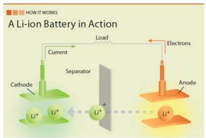
In a li-ion battery, positively charged lithium ions flow in a conducting electrolyte, through a separator, to the cathode. This leaves a negative charge of electrons on the anode. When charging, this flow is reversed.
