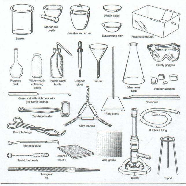
Beaker: glass or plastic; common sizes are 50 mL, 100 mL, 250 mL, 400 mL; glass beakers may be heated.
